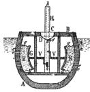
which can be screwed in toward the centerline to create a flooded chamber, and screwed out to expel the water and seal the opening.
